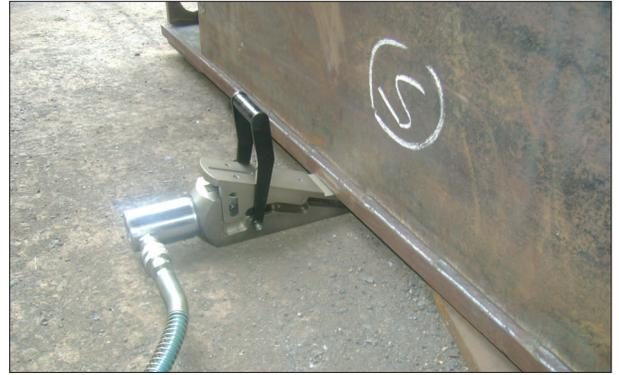
The HVW-10 has been developed as an easy to use / cost effective way to find solutions to heavy lifting where minimal clearance is available. It will lift objects vertically where an access gap of 3/8"(9.5mm) or more is available. The HVW-10 will lift an object fast, secure and safe with a lifting force of 16 Tons per tool. Multiple units can be used if greater lifting force is needed.
