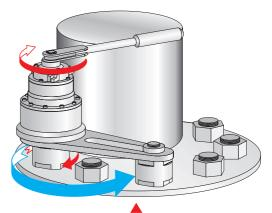
In this application, if it takes more than 180° to take up the wind-up at the required torque, this tightening operation will be impossible without an 'Anti Wind-Up Ratchet'.
