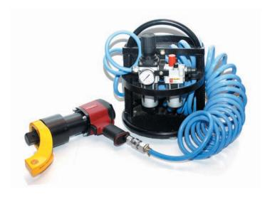
It is used to regulate the air pressure and properly lubricate the air motor for ultimate life. The Regulator regulates the inlet air pressure and controls the output torque of pneumatic torque wrench. All pneumatic tools must be used with FRL Unit. It is strongly advised not to exceed the maximum operating pressure as specified in the individual tool certificate.
