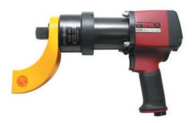
A Pneumatic Torque Wrench is an air motor driven planetary gear box having a very high reduction ratio. The gear box is provisioned with a reaction arm to absorb the torque reaction. Unlike impact wrench a pneumatic torque wrench is driven by continuous gearing and hence has no noisy and hazardous hammering. This is why a pneumatic torque wrench has an excellent accuracy and repeatability. Pneumatic torque wrench offers following significant advantages:
