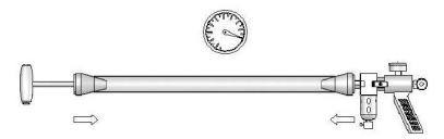
1) Connect air supply to the gun Plug both ends of the tube to be tested with Plugging 'T' handle one end and vacuum gun at other end.
